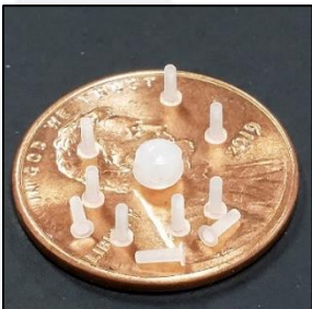
10 micro Plungers molded from a single pellet of resin
