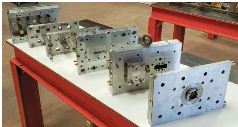
Matrix Tool has made its own mold bases and frames for decades, extending the precision of its cavities to the entire mold system.
