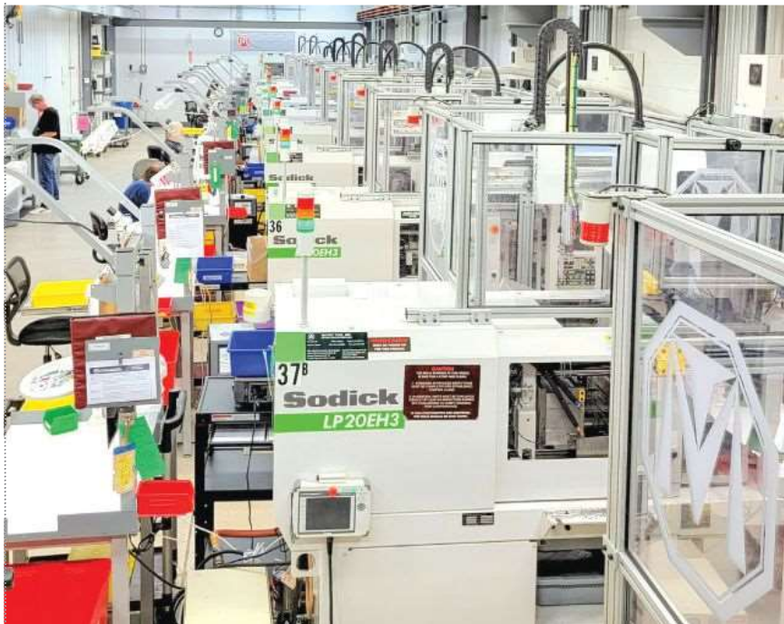
Matrix Tool's dedicated micromolding space runs 10 Sodick Plustech injection molding machines, eight of which have identical setups for seamless processing.
